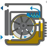
offers remarkable advantages, first among them being greater volume yield because the vanes are in constant contact with the inner wall of the stator and form a perfectly airtight seal with no leaks along the wall thanks to a continuous film of oil. In this type of compressor no axial thrust
