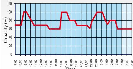
**Profile 3:** this profile represent an application with an eight-hour shift at constant consumption for five days a week. Air demand tends to stay around 90% of maximum requirement.
